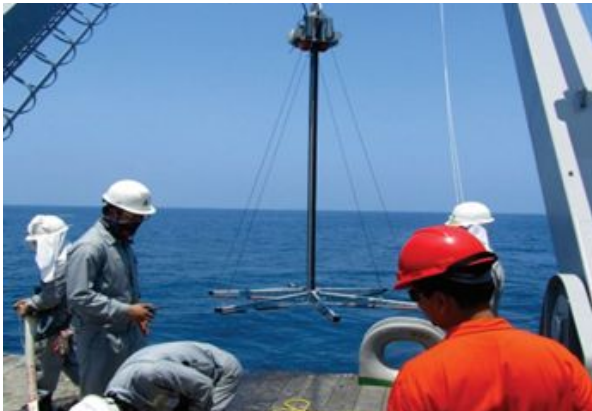
From the stern using the A-frame plus hoisting winch.
